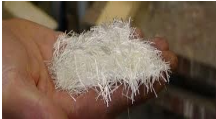
Figure:2.1 Glass fiber of size 7mm
